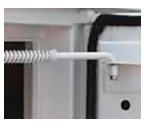
The spring-loaded door holder is on all vertical doors. It gives you easy access to your tools and gear by holding the door open in a 90-degree position. The hasp is removable when you need to have an extra-wide opening.
